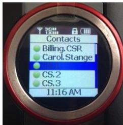
The image on the left shows the Contacts Screen. It lists all available contacts. To make a 1 to 1 Ad hoc call, use the side arrow buttons to move up or down the list, until you have highlighted the contact you wish to call. Then start the call by clicking the red PTT button. Hold that button down while you speak. This is called holding the floor.
